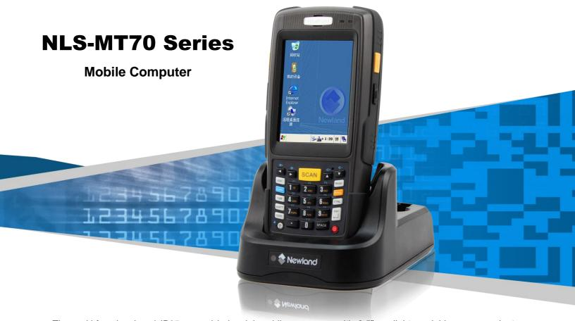
The multi-functional and IP65 rugged industrial mobile computer, with 3.5" sunlight readable screen, adopts Microsoft Windows CE.NET 6.0 operation system, as well as high-speed CPU of Marvell XScale PXA310 806MHz, 2GB large user flash memory and the module design provides convenience for customization. MT70 supports WiFi/Bluetooth/GSM/GPRS wireless communication, is quite suitable for applications such as warehouse, logistics, parking, delivery etc.
