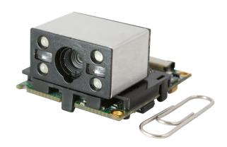
Designed for OEM applications, this high performance CMOS engine can easily be integrated into various solutions such as kiosks, ticketing machines, PDA's and many more.
