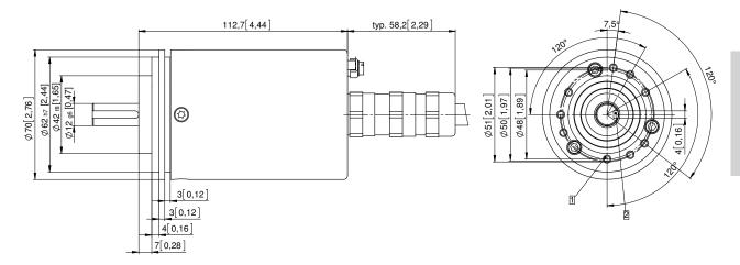
Clamping / synchronous flange, ø 70 [2.76] Shaft type 2 with radial cable outlet
