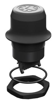
**Mounting**The Anybus Wireless Bolt is mounted into a 50.5 mm (M50) hole in the host device. The top ("helmet") goes on the outside and provides an IP67 exterior. The bottom is located inside the machine or cabinet (IP21).
